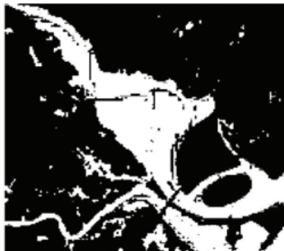
Figure 4: Distinguishing Water Areas from Non-Water Using NDWI
