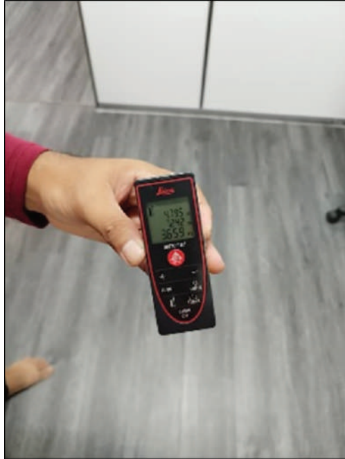
Figure 1.1 : Distometer to Measured the Dimension of Strata Parcel
