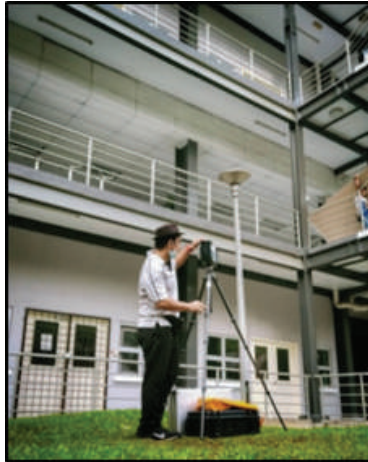
Gambar 1: Kerja imbasan TLS
